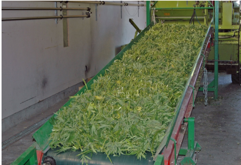
Figure 14. Green hemp decortication with a combine (ETH, 2006)
